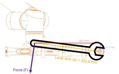
It is important to understand that the lever arm is only measured in the plane perpendicular to the tightening axis. In the example above, the distance of 173.3 mm (shown on the top image in green) in the direction of the tightening axis is not considered for the lever arm calculation.
