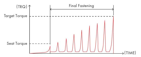
Some pulse-driven tools can reach tightening torques up to 150 Nm - 180 Nm, but accuracy of this torque may not be as high as a continuous tool, so they might not be suitable for some processes.
